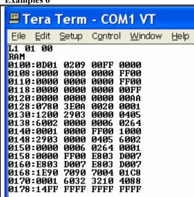
This example illustrates Cmd "L" which is used to show a 128 byte block of memory. The "1" that immediately follows the "L" indicates that the memory to be viewed will be RAM. The next two hex bytes are the beginning address. In this case, the example specifies a starting address of 0x0100, so 128 bytes [0x0100...0x017F] is shown.
