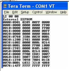
Another illustration of Cmd "L", but this time we are looking at a 128 byte block of the external EEPROM starting at address 0x0000.
