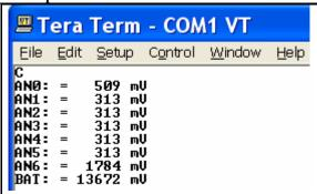
Here you see the measured voltages on the analog inputs (screw terminals labeled AN0..AN5) and the voltage on the voltage divider (AN6) that monitors the VBATT voltage. The AN6 reading is the actual measured voltage at the divider. The VBATT voltage is a constant times AN6 and this is shown as the reading labeled "BAT". All values are shown as decimal integers with millivolt units.
