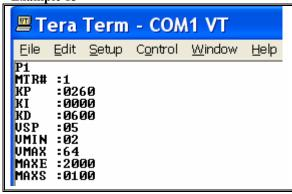
Here the "P" command is used to show you the parameters that affect PID operation of Mtr1. This command is also used to set the KP, KI, and KD parameters during "PID Tuning" of your motors for closed loop operation.
