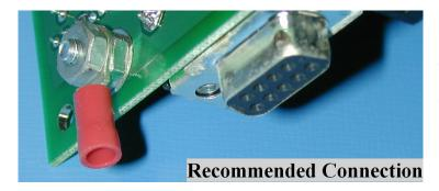
With power disabled, connect VBATT and GND wires to the board terminals using the supplied hardware (screws, double nuts, terminal lugs).
