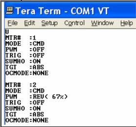
Cmd "U" is used here to show the status of both motors. Notice that the line labeled "PWM" for Mtr2 shows that the motor is now being powered in the reverse direction with a duty cycle of 67% as directed by the command of example 10.
