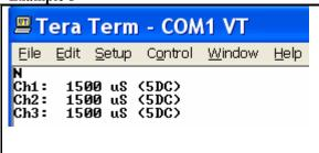
Cmd "N" is useful for verifying communication when using R/C to control the motor(s). It is also useful for transmitter switch tuning as explained in the Dalf Owner's Manual.
