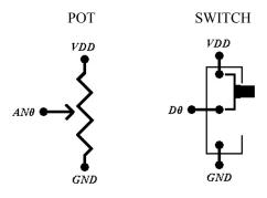
The control for the pot hookup for Motor2 is identical to that of Motor1 except it uses AN1. D1 is the motor direction input (POTF operating mode only) and has similar connections to that of the On/Off switch.
