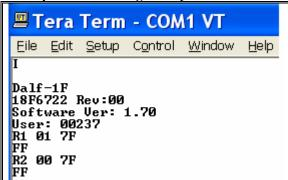
Here we again reset the board using the "I" command, but this time first **press and hold down on the push button labeled "BTN"** until after you see the greeting.
