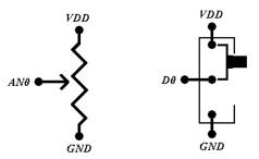
If PotF mode is used, connect the additional "Direction Control Switch" (Forward=VDD, Reverse=GND) to the D1 input on the Dalf board using a SPDT switch with similar hookup to that shown for D0.
