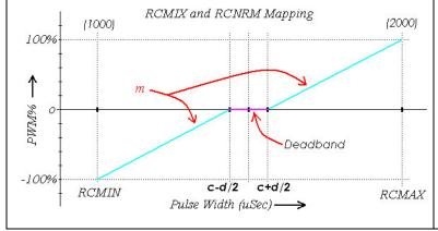
The R/C Pulse Width Measurement is mapped to a motor duty cycle % as illustrated.
