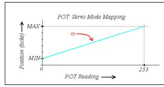
The POT Reading is mapped to a motor position as illustrated. The slope m is
