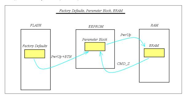
When you receive the board from the factory, the factory defaults will have been stored in the Parameter Block so that when the board is powered up it will use the defaults.
