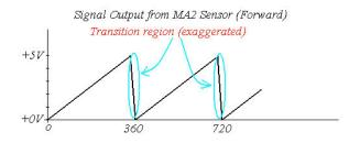
The ADC Module captures the sensor reading asynchronous to the motor movement.
