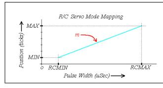
The R/C Pulse Width Measurement is mapped to a motor position as illustrated. A scaled value m is pre-computed and stored in RAM to minimize run time computation.
